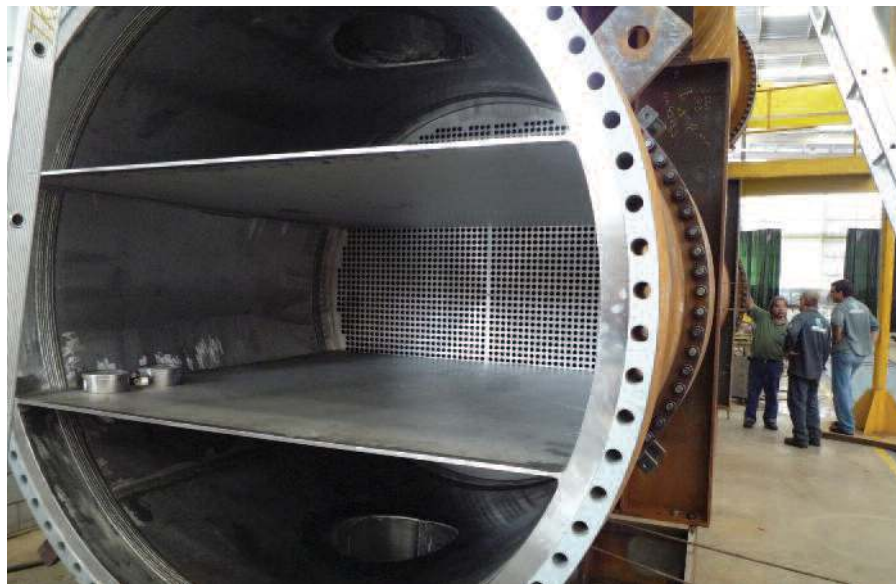
Fig. 9. A heat exchanger with clad tube sheet and shell. The base is carbon steel and the cladding is super duplex (Photo by SMT b.v.).
