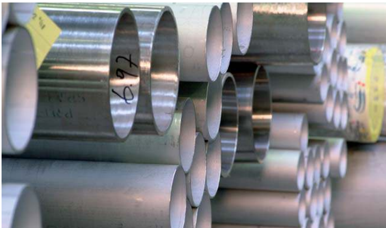
Duplex qualities are magnetic, but do not become hard. Because of the large chromium percentage and the presence of molybdenum the alloy has an excellent durability against all forms of corrosion such as stress corrosion cracking.
