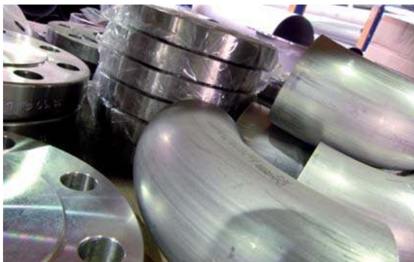
If chromium is alloyed in steel, than it appears that a content of 12% of chromium is enough to form a layer of chromic oxide on the steel surface, through which passivation appears.
