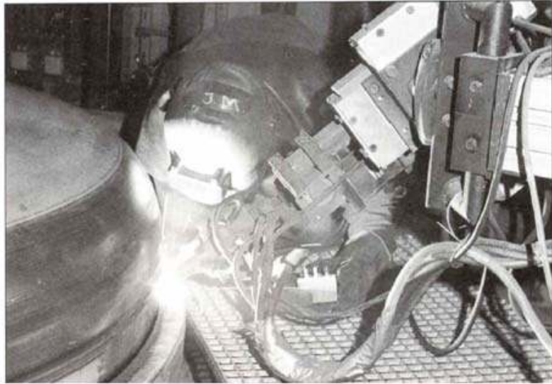
GMAW weld of a stainless steel cover
