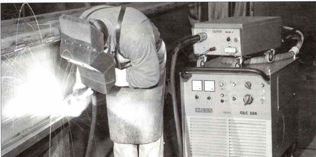
GTAW welding of a stainless steel tube
