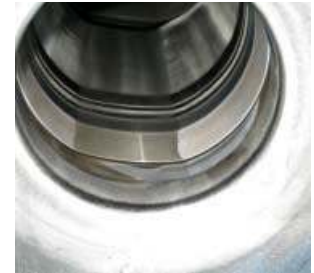
Left: Red-brown Rouge layer in WFI-tube system (material 316L)
