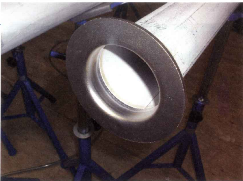
Picture 3. A smooth and perfect root penetration can be seen on the transition between the pipe and the collar. This photo was taken at Hamer Installatietechniek immediately after welding without post-treatment.
