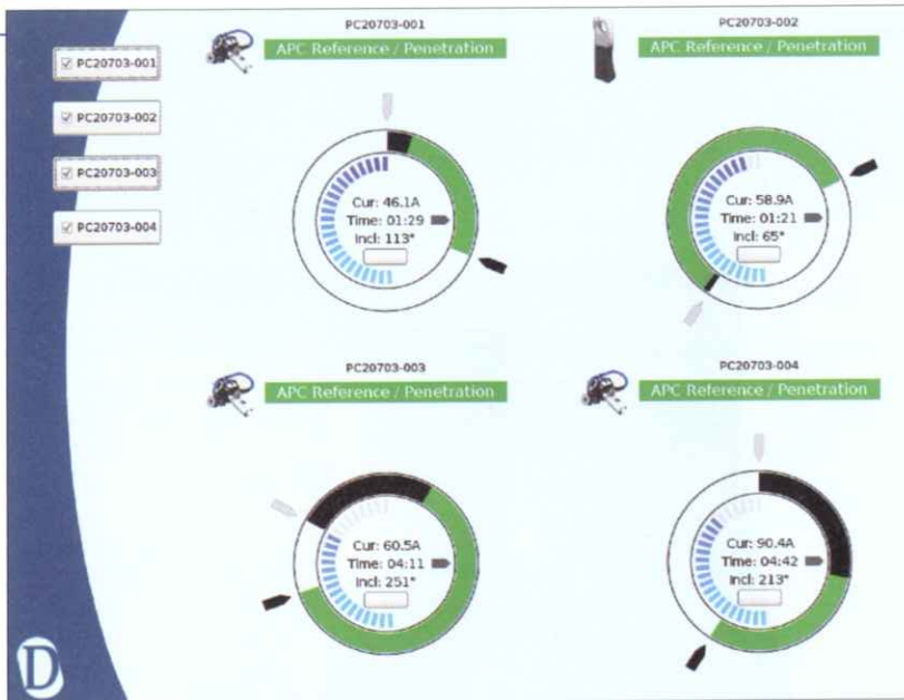
Picture 4: Weldclock, with the progress of four root penetrations and other weld information visible in real-time on the touch screen.
