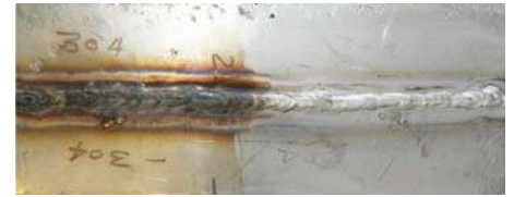
Image 9. The right half is nearly free of iron bonds which makes it look as if it has been pickled (photo: Poligrat).
