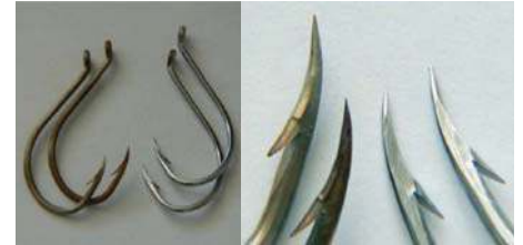
Image 10. Untreated AISI430 fish hooks, treated fish hooks on the right (source: Poligrat)
