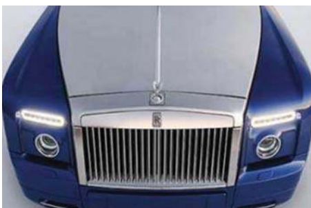
Image 6. AISI304 motor cap treated with Polinox Protect after four years of use.
