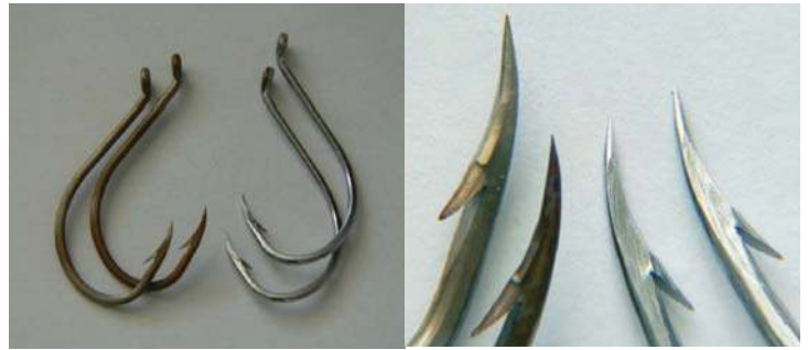
Image 10. Untreated AISI430 fish hooks, treated fish hooks on the right (source: Poligrat)
