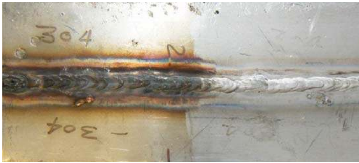
Image 9. The right half is nearly free of iron bonds which makes it look as if it has been pickled (photo: Poligrat).
