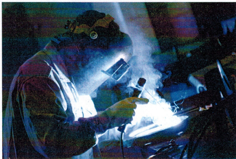
As a general guideline, when welding stainless steel grades, any additional materials need to have, as much as possible, the same chemical composition as the parts that have to be welded.
